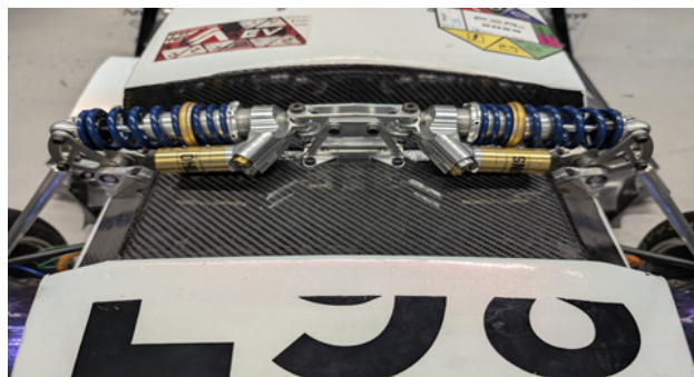
Figure 11: Inboard front suspension of the HPF025 race car with twin coilover dampers and rocker linkage; the bracket subject to optimization interfaces to the chassis in the middle via a four-bolt pattern.
